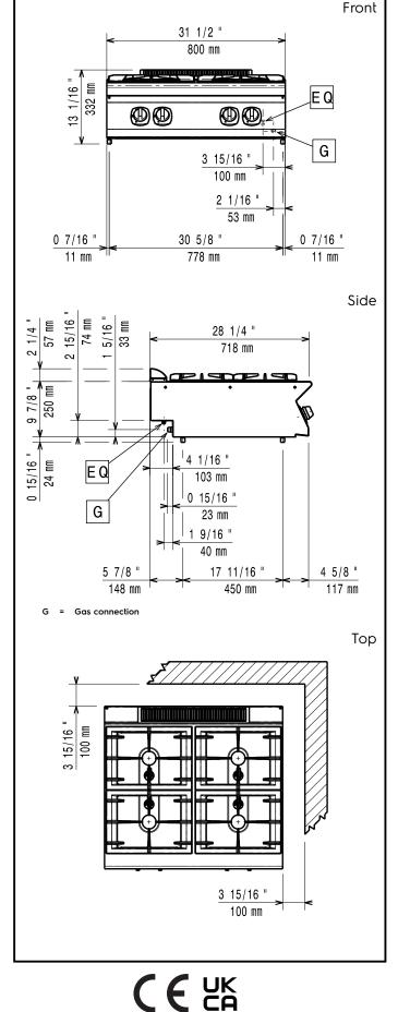
Modular Cooking Range Line 700XP 4-Burner Gas Boiling Top
